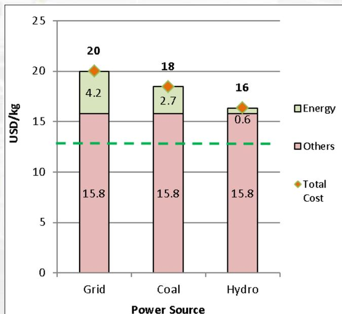
Figure 3: Effect of Energy Costs on Polysilicon Manufacturing Costs in India
