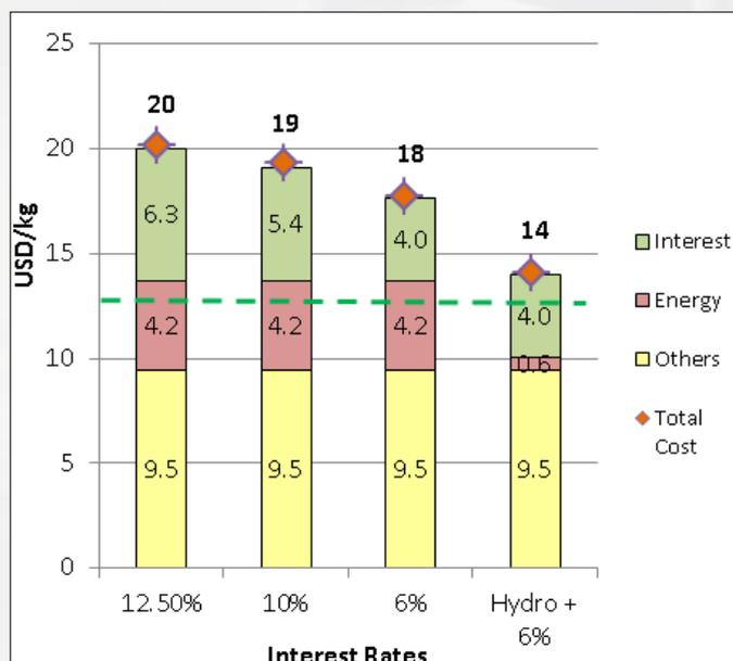
Figure 4: Effect of Interest Rates on Polysilicon Manufacturing Costs in India
