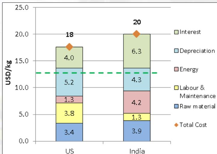
Figure 2: Cost Break-up of Polysilicon Manufacturing
